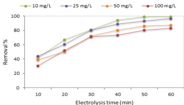
**Figure 3:** Effect of reaction time and concentration on the TC removal efficiency ( $d=2.5$  cm,  $t=60$  min,  $C_0=10$  mg/L, Voltage = 60 V, current density: 400 A/m<sup>2</sup> and pH=6).
