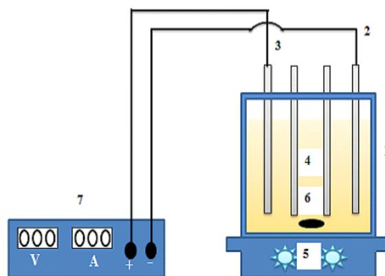
Figure 2: Bench-scale EC reactor with bipolar electrodes in parallel connection.
