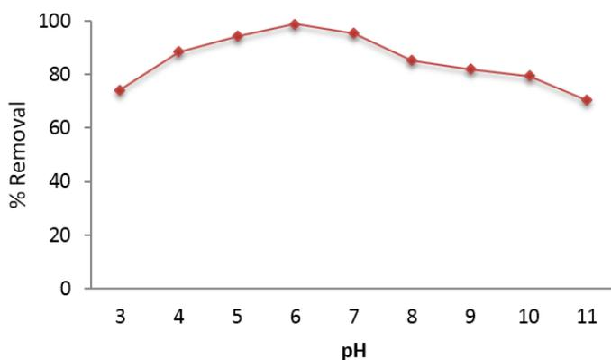
**Figure 5:** Effect of pH on removal efficiency of TC ( $d=2.5$  cm,  $t=60$  min,  $C_0=10$  mg/L, Voltage = 60 V, current density: 400 A/m<sup>2</sup>).
