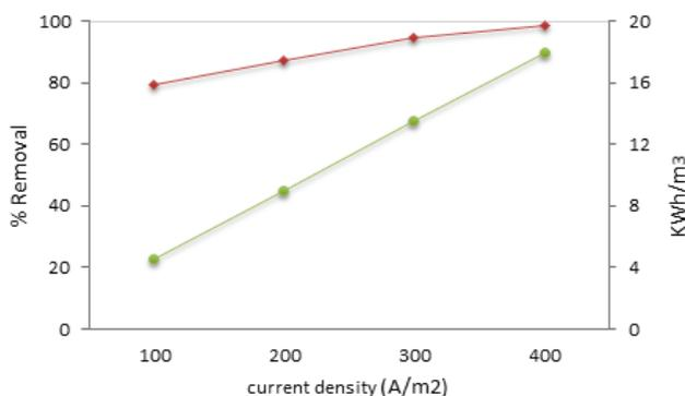
**Figure 4:** The effect of density and its effect on electrode consumption ( $d=2.5$  cm,  $t=60$  min,  $C_0=10$  mg/L, Voltage = 60 V, pH=6).
