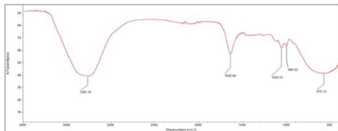
**Figure 4: FTIR Spectrum of CIS.**
