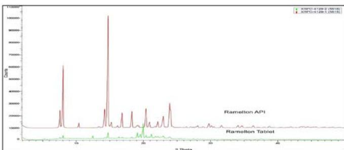
**Figure 7:** Overlay XRD diffractogram of the Ramelteon API and the finished dosage form.
