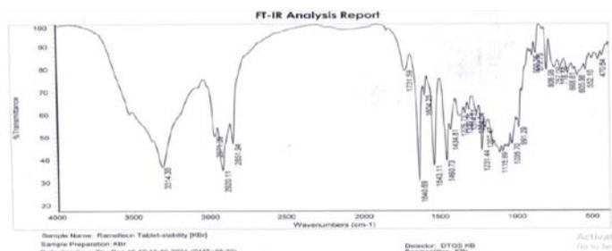
**Figure 2:** FTIR spectrum of the Ramelteon tablet - Physical mixture samples. Y axis represents % Transmittance and X-axis represents wave numbers (cm<sup>-1</sup>).
