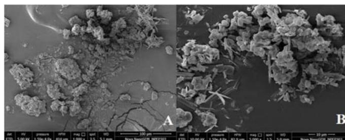
**Figure 4:** Field Emission Scanning Electron Microscopy of DCH1 formulation. a) Particles with size range 5-50µm range b) Drug found to be embedded in the polymer after spray drying.
