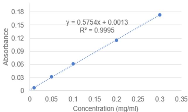
Figure 2: Calibration curve of zinc sulfate.
