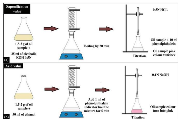
**Figure 1:** Schematic representation of physicochemical analysis performed. (a) Saponification value (b) Acid value.
