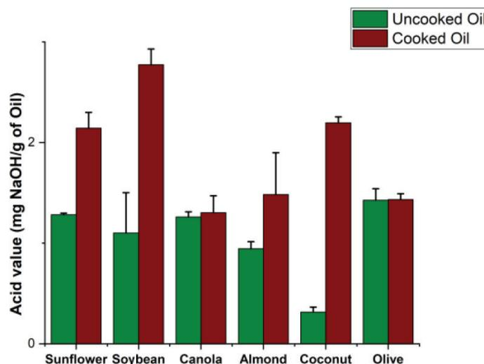
**Figure 3:** Acid values of oil samples before and after cooking.
