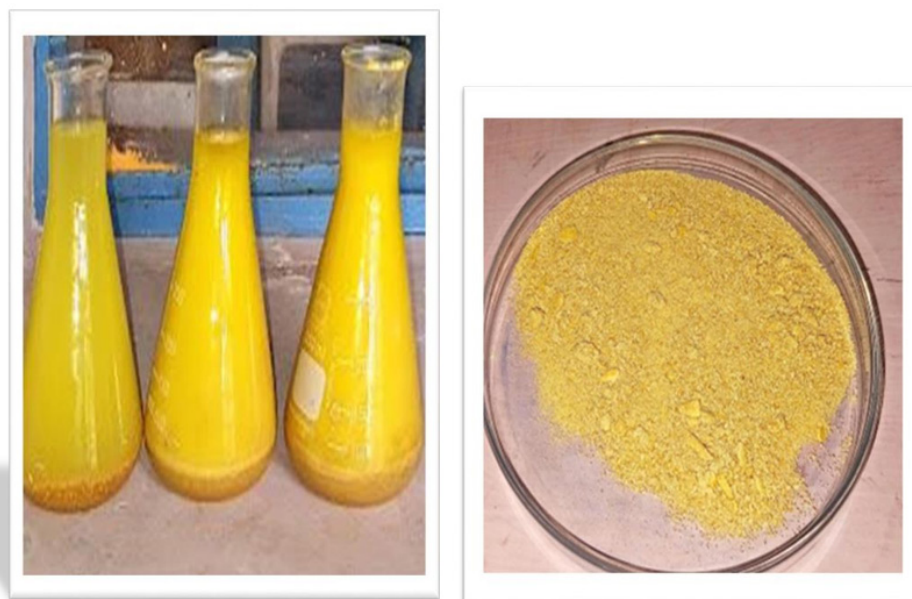
Figure 1: a and b Extraction of fenugreek seed in ethanol and dry powder.
