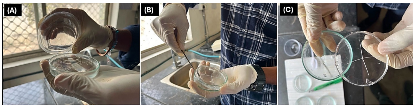
Figure 2: Images show that fabrication of microchannels by using ABS. Image (A) shows 10:1 ratio of PDMS and crosslinker mixture was poured on the petri dish mould in which ABS filament is there. Image (B) shows the PDMS was solidified by keeping the liquid mould in hot air oven for 1 hr at 60°C. After the solidification the PDMS is peeled off from petridish. Image (C) shows fabricated ABS based PDMS microchannel.
