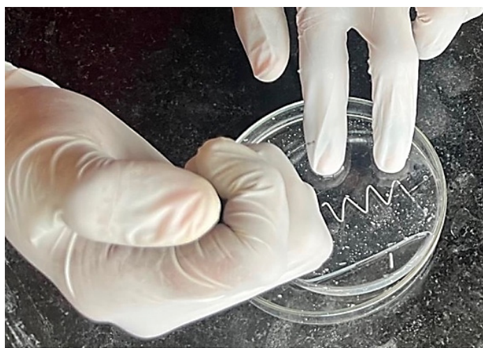
Figure 3: Image shows that removing of ABS using acetone. Acetone was injected from on nozzle forcefully, then acetone dissolves ABS which was pumped out from other nozzle.
