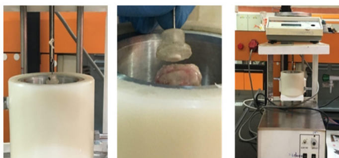
Figure 2: Mucoadhesive strength testing apparatus.
